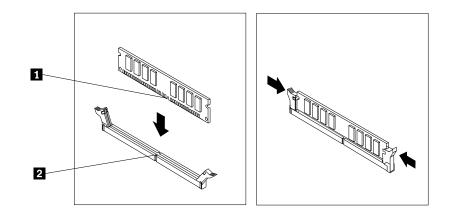
Figure 16. Installing a memory module
